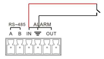
**Example 1**: You want to use Input 1 Alarm and trigger recording Channel 1 only when alarm is normally close
