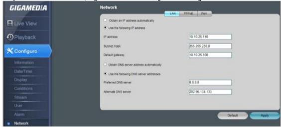
In this menu you will have to configure the new IP address of the camera and press Apply:
