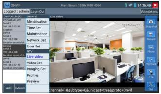
Snapshot: Click "snapshot" to save the current image as a JPEG file on the SD card
