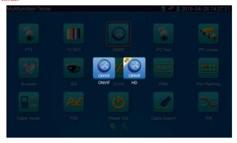
If you select ONVIF Rapid mode, the meter automatically scan different network segments for ONVIF cameras. It lists the camera name and IP address on the Device List. Tester can auto login camera and display camera image.
