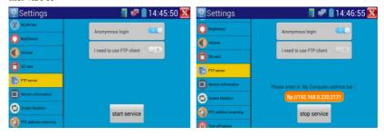
Start the FTP server and then input the tester's FTP address in the PC's address bar. This will enable the PC to read, copy and edit the files from the SD card without the use of SD card reader.
