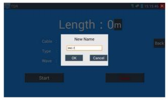
**Application:**TDR test is the use of pulse reflection method, to transmit pulse signal for tested cable, when cable is disconnected or short-circuit, reflected pulse is generated, the tester receives and deals with the reflected wave, measurement results displayed on the screen. TDR cable test can test cable length and short circuit, help engineer quickly find the cable's problem location. It is more convenient and efficient to repair the faulty cable.
