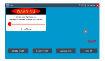
VFL four status can select—"Steady mode", "Evasive 1Hz", "Evasive 2Hz"and "Time off". Click button "Steady mode" to enter steady status, click button "Evasive 1Hz" and "Evasive 2Hz, to enter pulse mode, click button "Time off", VFL be turned off. Timed turn off can select (5mins, 10mins, 30mins, 60mins and 120mins).
