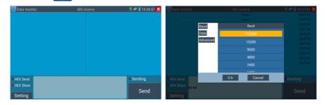
Click "Setting" to choose the baud rate of RS485/RS232; it must be the same as the DVR or the Control keyboard. The DVR or Control keyboard send the code to the tester, if it can be read, the protocol will shown on the upper right, like Pelco D, if not, like P:---
