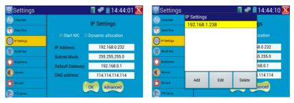
After setting an advanced IP address (refer to above photos), the tester can test two network segments (192.168.0.0) and (192.168.1.0).
