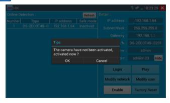
Hikvision activation: When connect the unactivated Hikvison camera to the tester, it will auto identify and display "Unactivate" at safety mode. Select needed activate the camera, click bottom right corner button "Enable", pop-up "the camera is not activate, activate now"?
