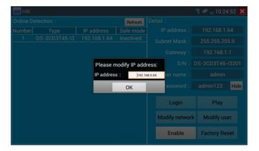
For other operations need login activated camera, when login, select the camera at the left "online detection", and input username and password to login.
