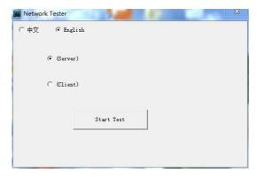
Tester as Client, tester's IP address is:192.168.0.230. The Server and the Client are at the same network segment, but with different IP address. Input Server's IP address 192.168.0.89 in the tester and click "Start" to test network bandwidth.
