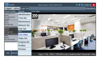
**IP camera video settings:** Click "Video Set" to enter the IP camera's encoder and resolution settings. Make the desired changes and click "OK "to save.
