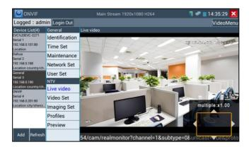
When the image is enlarged, if not operate on touch screen, it can operate by the keyboard ,press the key  $\begin{tabular}{l} TELE+ \end{tabular}$  to zoom in , press the key  $\begin{tabular}{l} WIDE- \end{tabular}$  to zoom out ,press upward and downward key to move image .
