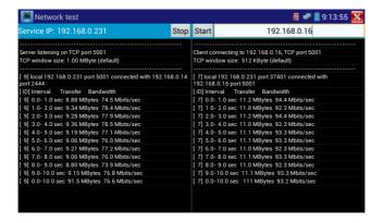
Network bandwidth testing can also be tested with a computer using compatible network bandwidth
