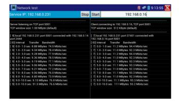
Or tester as a Server, computer as test Client (select Client,input tester's IP address to test)
