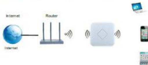
3. Gateway: Supply WAN connection from DSL, Cable Modem or broadband mobile phone network through PPPoE, Static IP, Dynamic IP
