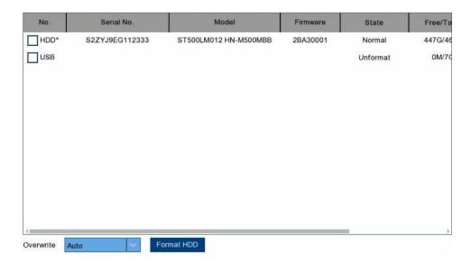
If the HDD is installed in the NVR for the first time, it must be formatted. Select the HDD and then click **Format HDD** button to format the HDD.
