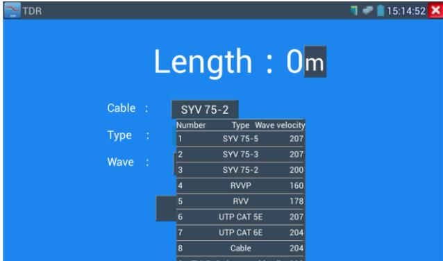
**User-defined calibration:** Choose the cable 100 meters to 200 meters (more than 50 meters), click “Cable”, “Type” to select user-defined 1 for calibration, 11 groups user-defined can be set.
