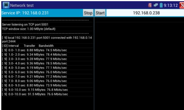
**b).Start send packet test:** Using the other IP tester, and type in the Server's IP address at the top right corner of the screen. This app is used to send packets for network speed testing. Click the “Start” button to send the packets and start testing.
