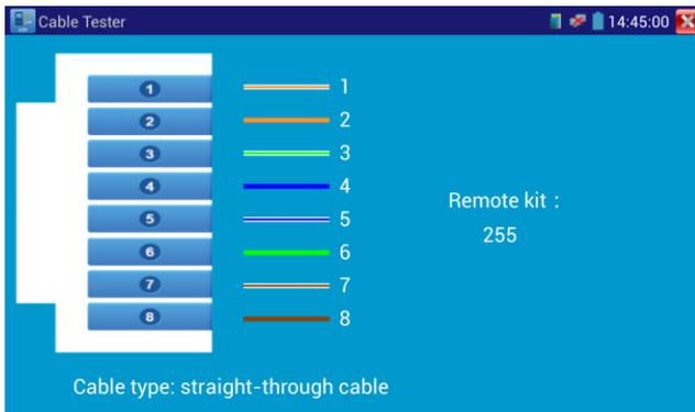
Test LAN cable or telephone cable.
