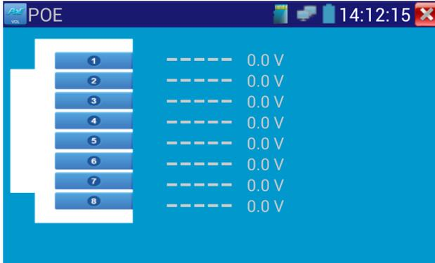
Connect a network cable from a PoE switch to the IP tester 's PSE IN port. Connect an IP camera or other PoE using node to IP tester's LAN port, the PoE voltage and the cable's pin connection status show on the screen.
