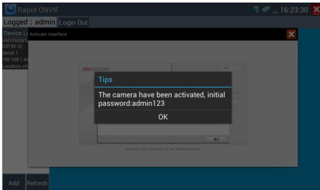
Back to Rapid ONVIF function, click log in to display the camera image ,the activation of HIKVISION Camera was completed .
