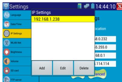
After setting an advanced IP address (refer to above photos), the tester can test two network segments (192.168.0.0) and (192.168.1.0).
