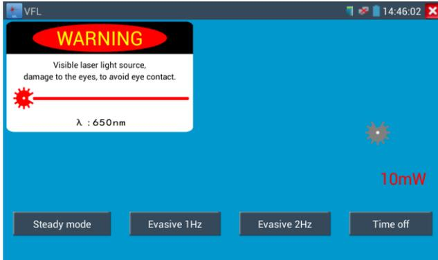
VFL four status can select——“Steady mode”, “Evasive 1Hz”, “Evasive 2Hz” and “Time off”. Click button “Steady mode” to enter steady status, click button “Evasive 1Hz” and “Evasive 2Hz” to enter pulse mode, click button “Time off”, VFL be turned off. Timed turn off can select (5mins, 10mins, 30mins, 60mins and 120mins).
