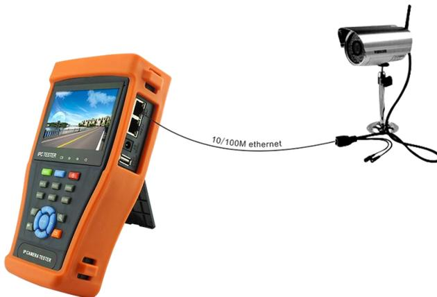
**Note:**1) If the IP camera requires PoE power, then connect the IP camera to the IP tester's LAN port . The tester will supply PoE Power for the IP camera. Click on the icon labeled POE to turn the PoE Power off or on.
