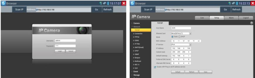
The IP camera and IP tester be on the same network segment for the browser to interface with the camera. If they are not in the same segment, click the button
