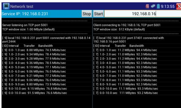
Or tester as a Server, computer as test Client ( select Client,input tester’s IP address to test)
