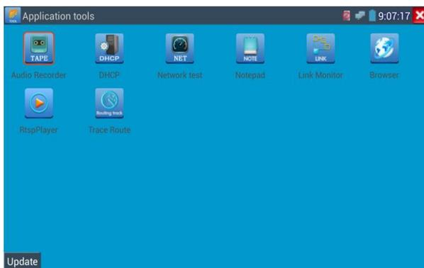
**Audio Record:** Connect an audio device to the IP tester's audio input port. Click the
