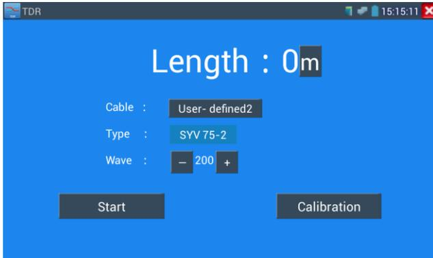
1. Select user-defined and click “Calibration” to enter test , click “user-defined 1” can define cable name, such as: AiPu BNC-5
