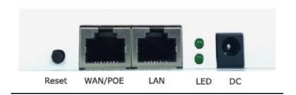
**DC**: Power Supply used for 12v/1A (optional)
